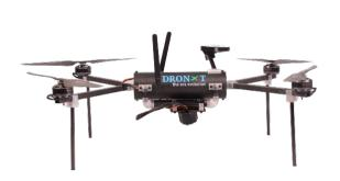
Rodnxt-S6, the first flagship multirotor UAV developed by Dronxt for surveillance missions delivers a strong 40 mins of operational endurance in a completely loaded configuration. With an innovative monocoque rugged airframe structure, it holds up heavily against adverse weather and terrain conditions.
